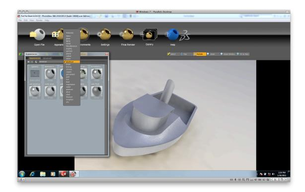
To make a part of your model a certain material, drag and drop your material onto the part of model you want to change – in this case, we chose Blue Anodize for the top of the boat:
